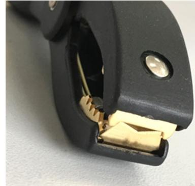
The BU-111STG is the high clamp force version of the BU-111 mid-size Kelvin battery clip (jaws electrically isolated). Used for accurate electrical impedance measurement.
